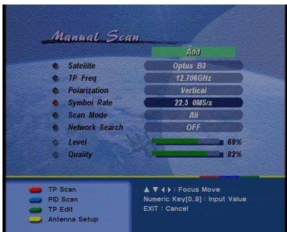
STEP 9 Go down to Symbol Rate and enter 2 2 5 0 0
