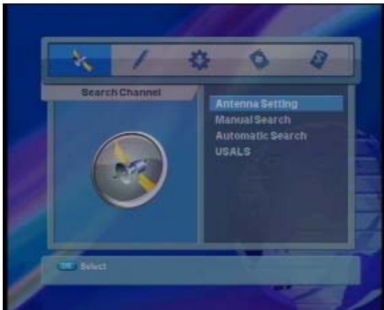
STEP 1 On the Arion Remote press "Menu" button. When the screen comes up. Using the lower arrow go to Manual Search
